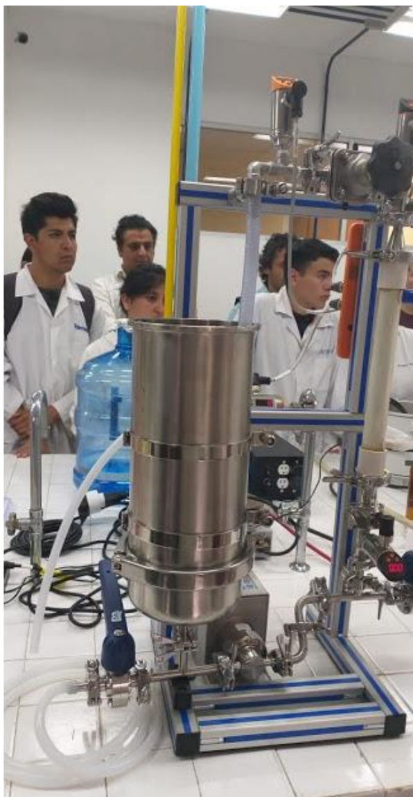
Experimental work at Pilot-plant scale facility demonstrating the use of equipment for the extraction / purification of phyco-pigments
