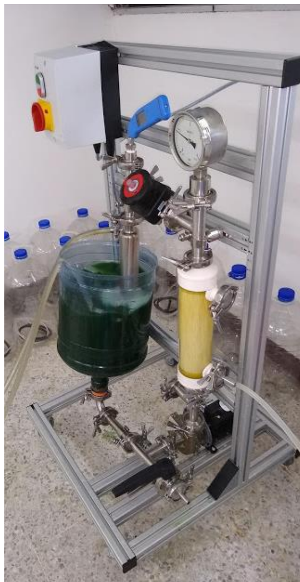
Experimental work at Pilot-plant scale facility demonstrating the use of equipment for the extraction / purification of phyco-pigments
