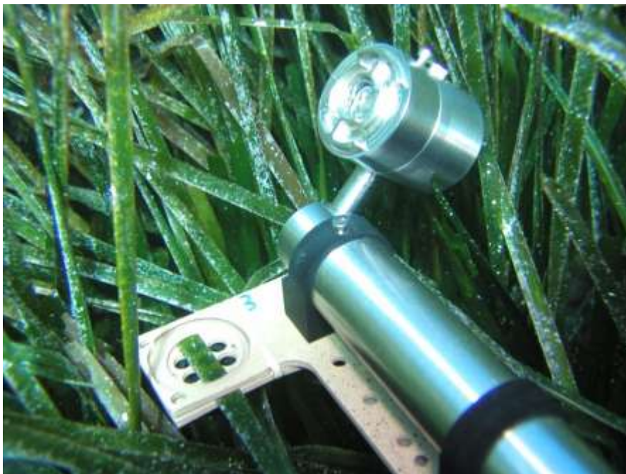
Shutter Fluorometer measuring Posidonia oceanica in the Mediterranean.
